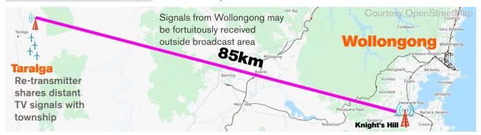
The Taralga wind farm re-transmitter receives a distant, fortuitous signal from Knight's Hill in the Illawarra area (85km away) for all free-to-air channels. The Taralga Wind Farm re-transmitter then re-broadcasts these channels to a small area, including most of Taralga township.
